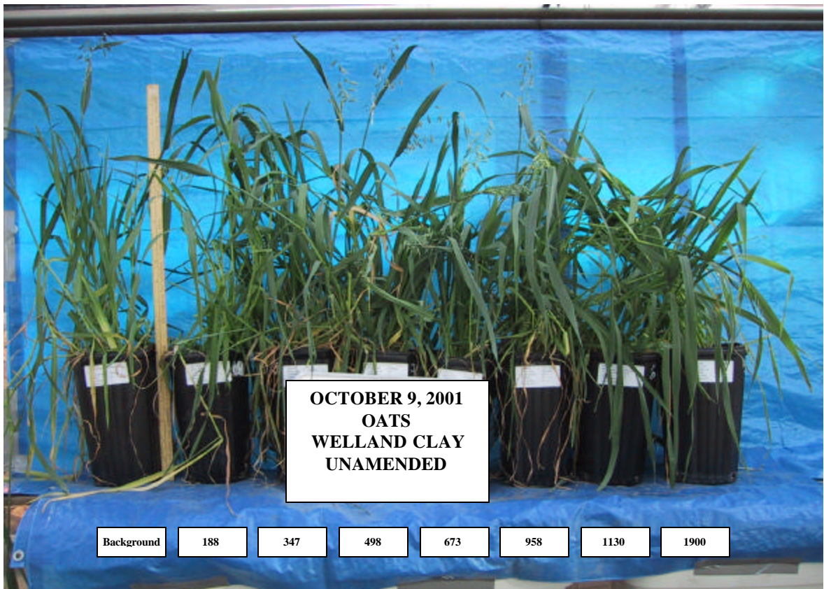
Plate 21: Oat on unamended Welland clay soil: Background to 1900 mg Ni/kg (at harvest)
