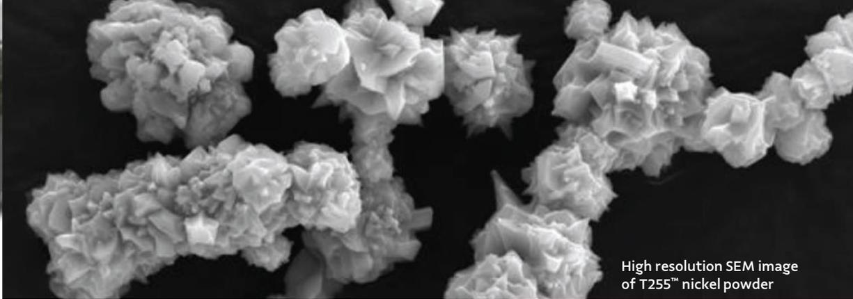
High resolution SEM image of T255™ nickel powder
