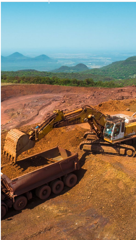
Ore extraction and transportation iron in the Santa Cruz mine, in Corumbá (MS). Photo: Ricardo Teles.
