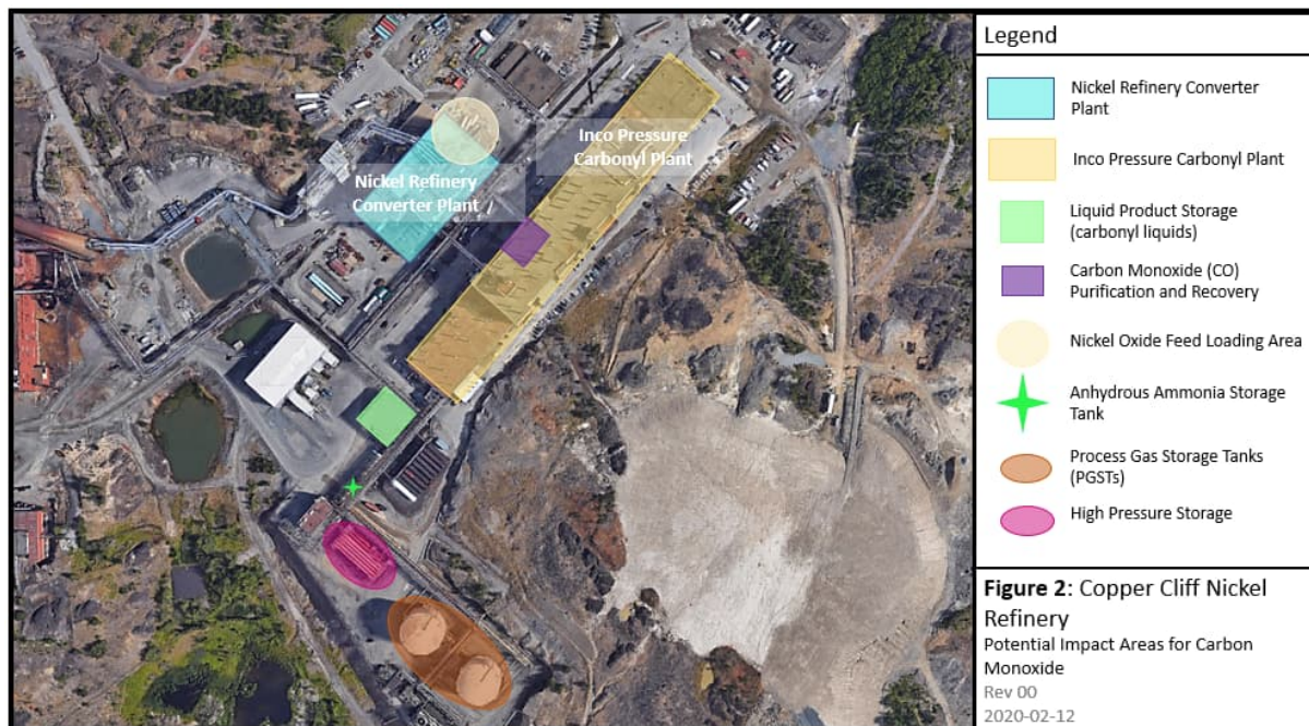
Figure 2 Location of Each Substance at CCNR
