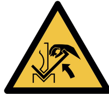
Hand Crushing between press brake and material
