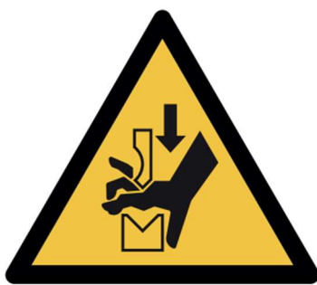
Hand Crushing between press brake tool
