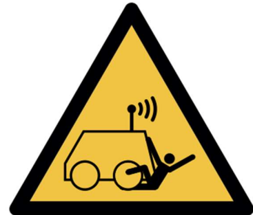
Run over by remote operator- controlled machine
