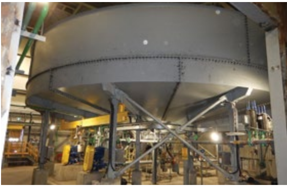
Dewatering of slurry begins in the thickener (left) and is completed in the filter press (right).
